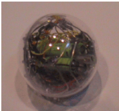
Figure 4: The smart ball developed for the LEGO Mindstorms RoboCup Jr.'99. © LEGO Lab 1999.
