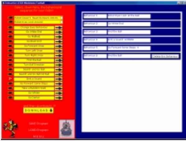
Figure 2: The programming environment. On the left is displayed all the primitive behaviors that the user can select to put on the right side in the control program. To the left of each primitive behavior is shown a small video camera icon. When clicking this icon, a small video sequence will display the robot behavior. © LEGO Lab 1999.
